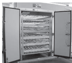
Fig.3 花芽誘導装置 Fig.3 Floral bud induction system
